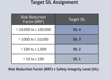
A Safety Instrumented Function (SIF) is required when the level of risk reduction offered by existing protection layers does not achieve a tolerable residual risk. A **Safety** Integrity Level (SIL) will be assigned depending on the additional risk reduction
