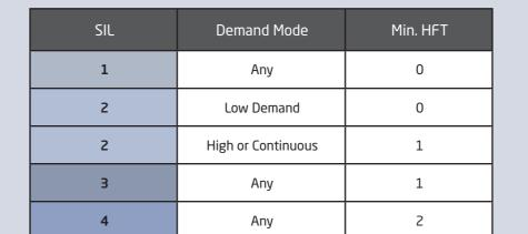
Various system architectures can be employed to meet the **Architectural Constraints or** IEC 61511 Clause 11.4.3 states that HFT must comply with IEC 61508 route 1H or IEC 61508 Route 2H / IEC 61511 clause 11.4.5 to 11.4.9
